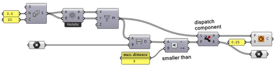
In this exercise, points are filtered out gradually over distance. The further away, the more points will be filtered out.
